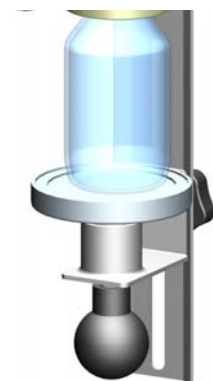
adjustable bottle support, spring loaded plate
